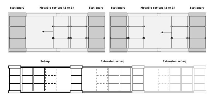
One UBeTrack<sup>TM</sup> can consist of 2 or 3 mobile shelves. The total width can vary, see the illustration below. This can be increased in O  $^{63/64}$  inch increments up to a maximum of 9  $^{27/32}$  inch which in turn alters the width of the walkway.
